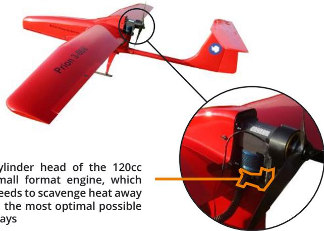
Cylinder head of the 120cc small format engine, which needs to scavenge heat away in the most optimal possible ways
